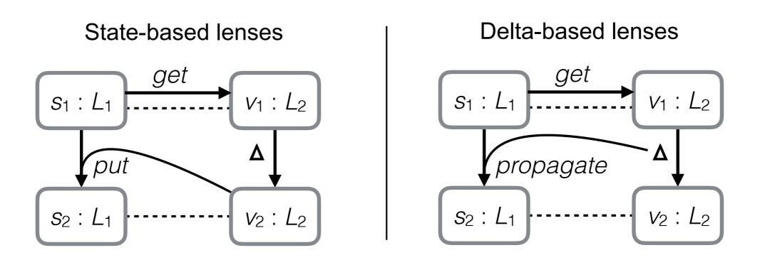
In the first (more basic) BX pattern, *get* maps a source to a view; *put* maps back a changed view to a source while taking into account the original source so that BX can go beyond bijective functions. In the second (more detailed) BX pattern, *put* has been replaced by a decomposition of differencing and change propagation.
