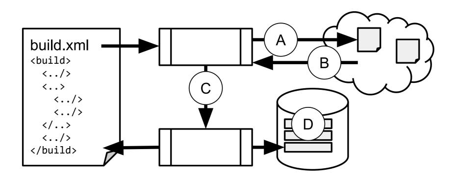
A depiction of data flow and related transient states. A and B represent web request and response, respectively, C depicts piping of program output, and D shows transient data in memory or database.
